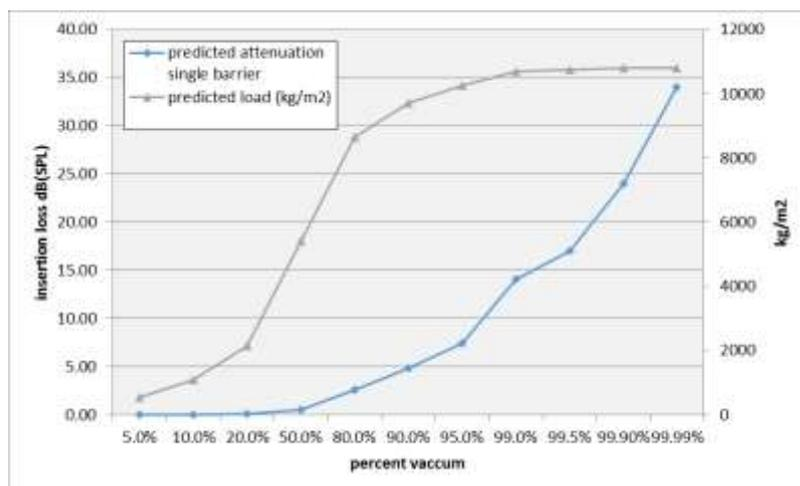
Figure 1 - predicted insertion loss and mechanical load
