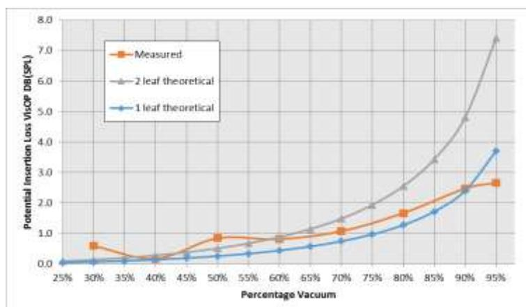
**Figure 8 - final relationship, measured VS predictions**
