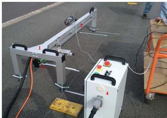
Figure 2 – 3D Surface texture equipment 1: Chassis – 2: Motorized axle – 3: Brushless motor – 4: Control unit
