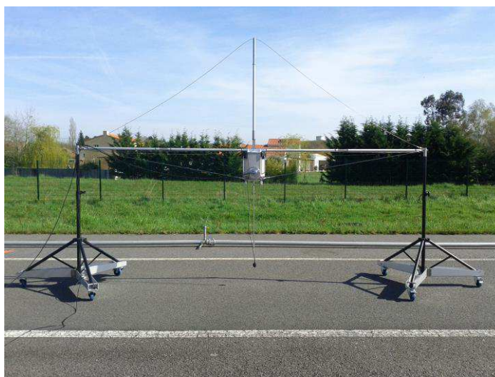
Figure 5 – Absorption coefficient measurement according to ISO 13472-1 Standard. Experimental device installed on the Ifstar reference test track
