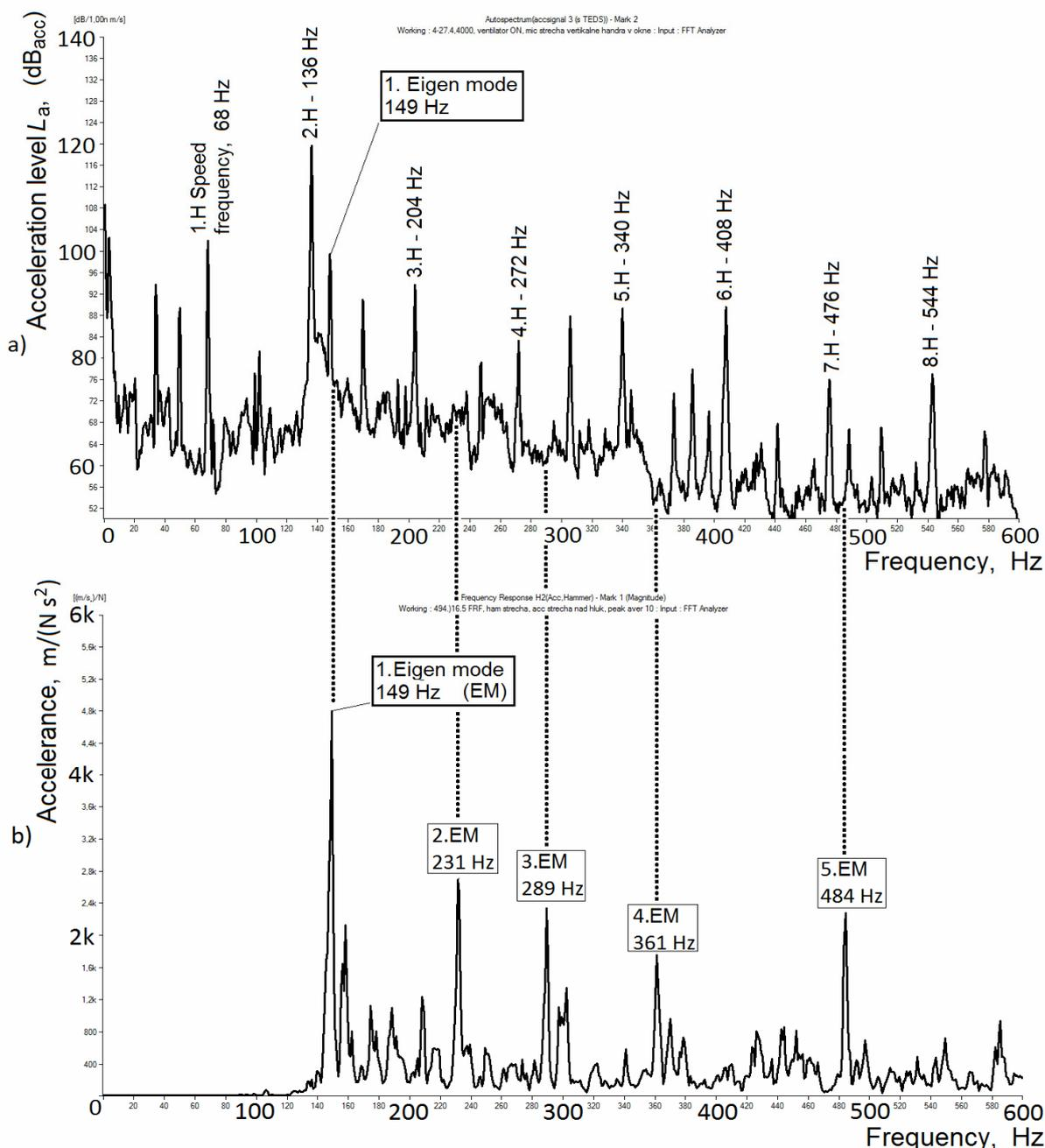
Figure 2 –a) FFT analysis of a subtle structure (car body) at a given rpm of the combustion engine; b) Eigen frequencies the modal analysis of the same subtle structure
