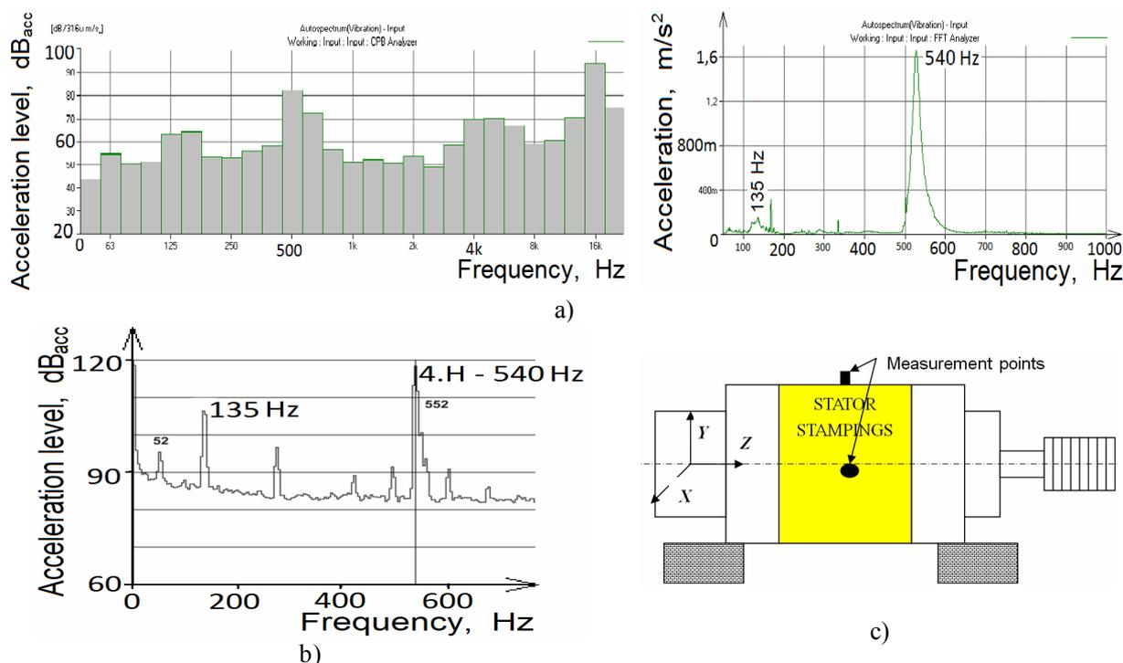
Figure 3 – a) Frequency spectrum and Eigen frequency (right) during freewheeling at specific electromotor revolutions; b) Measured frequency spectrum; c) Scheme of the electromotor
