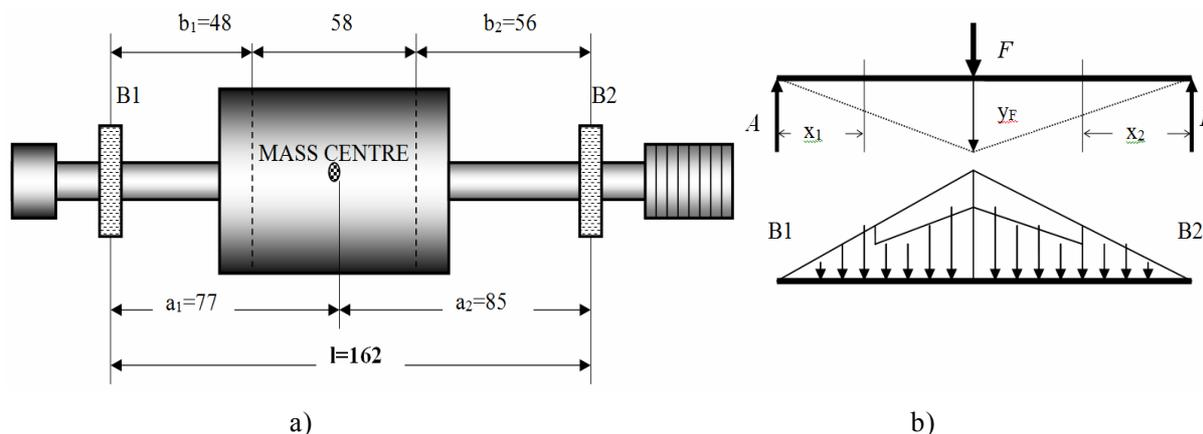
Figure 4 – a) Schema of the electromotor rotor; b) Schema for the calculation of shaft stiffness along the axis of rotation
