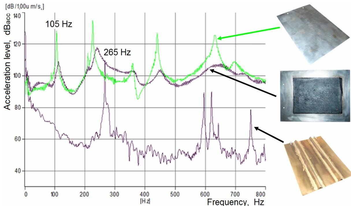
Figure 6 – Comparing the frequency spectrums of a non-damped subtle structure with a damped subtle structure utilizing resilient material (VIBROFOL) and by tuning of the structure
