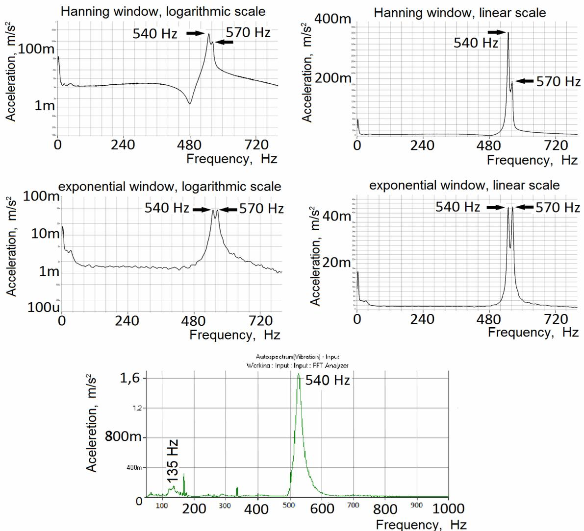
Figure 5 – Eigen frequencies from the modal analysis of the electromotor by using Hanning and exponential window for scale logarithmic (left) and linear (right). Frequency analysis of the electromotor in linear scale (bottom)
