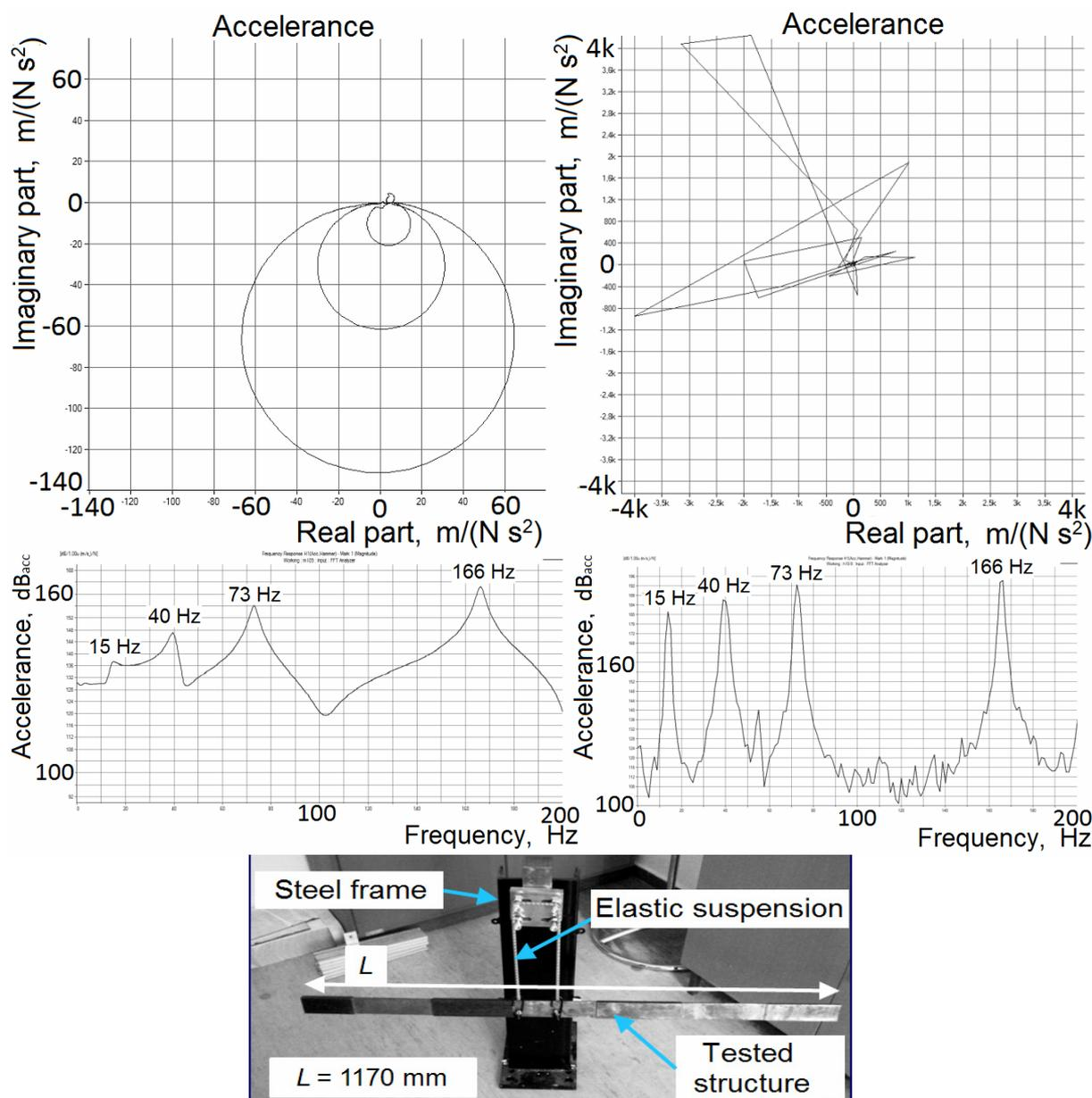
Figure 1 – Nyquist polar diagram and transmission function utilizing the exponential window (left) and Hanning window (right) for impact excitation of a suspended beam (down)
