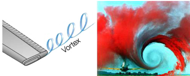
Figure 2: Air turbulences from an aeroplane wing tip; after NASA (2)
