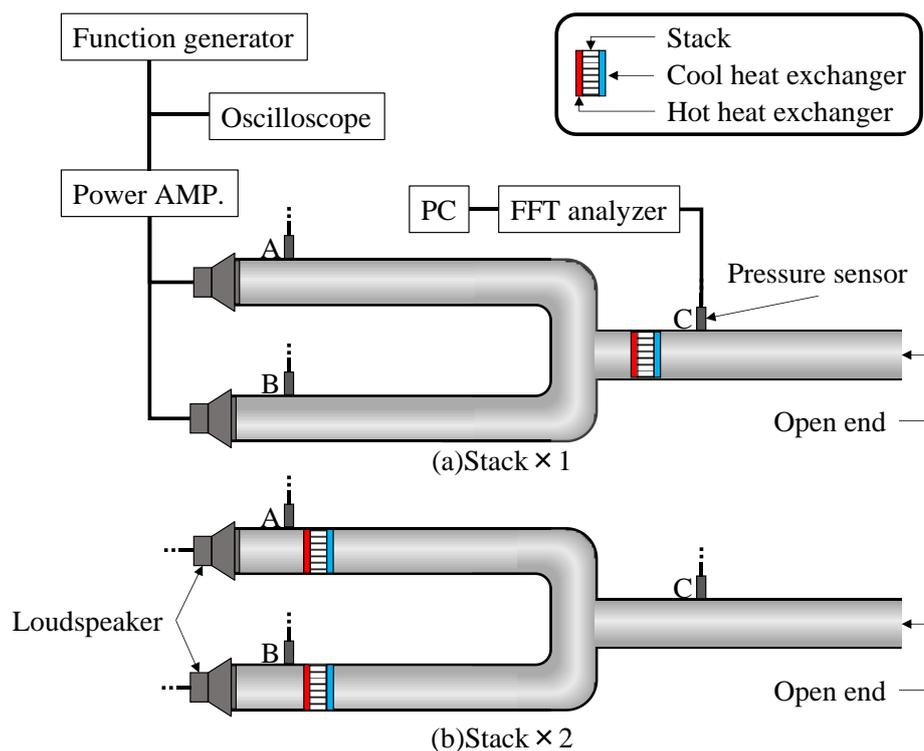
Figures 1(a), 1(b) Experimental setup with muffler of a multi-cylinder engine. Figure 1(a) shows the condition of stack was installed on back of the confluence. Figure 1(b) shows the condition of stack installed in front of the confluence.
