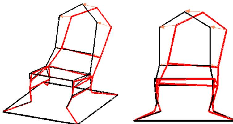
Figure 4 Lateral vibration mode shapes
