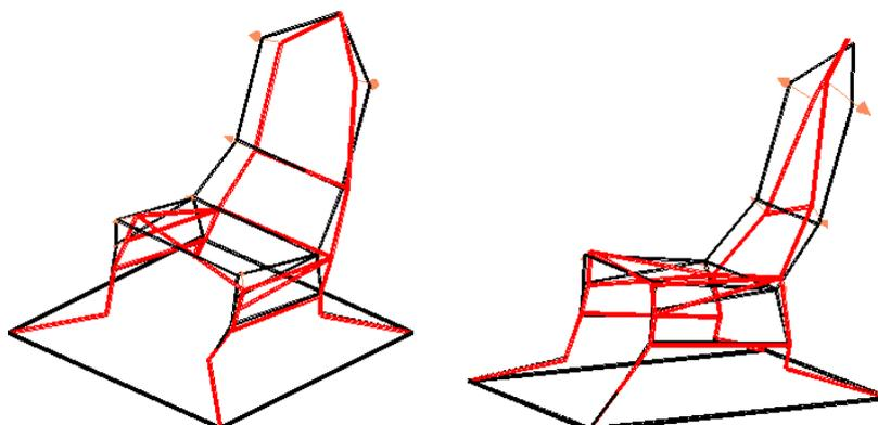
Figure 6 Twisting vibration mode shapes
