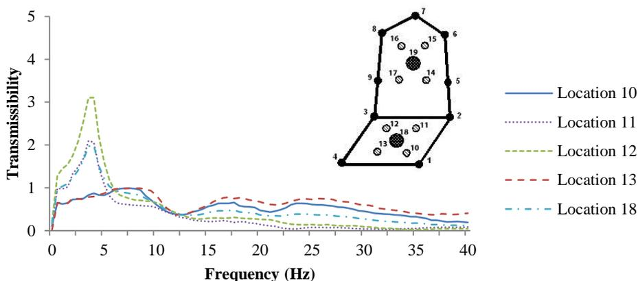
Figure 15 Vertical transmissibilities at measurement locations on seat cushion surface.
