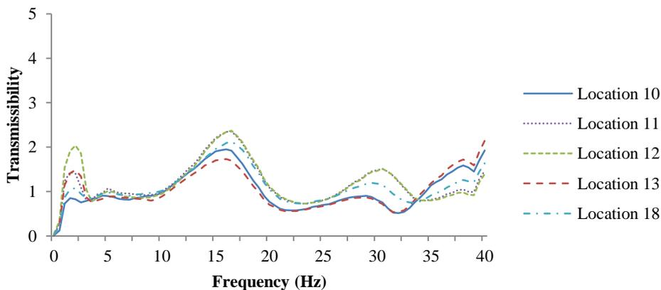
Figure 14 Lateral transmissibilities at measurement locations on seat cushion surface.
