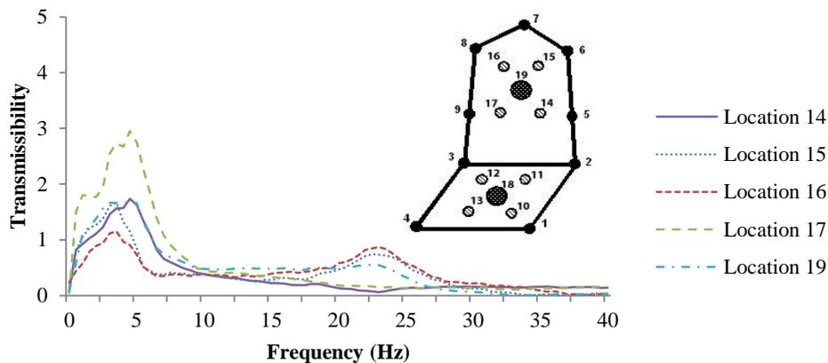
Figure 10 Fore-aft transmissibilities at measurement locations on seatback surface.
