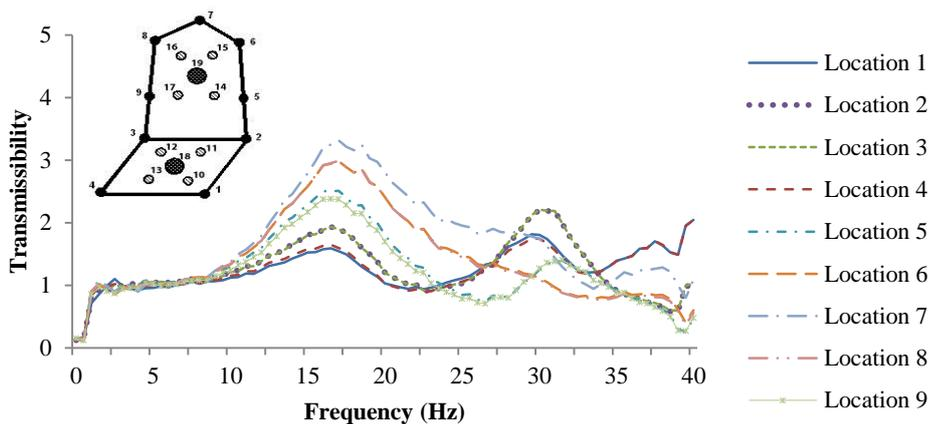
Figure 8 Lateral transmissibilities at measurement locations on seat frame
