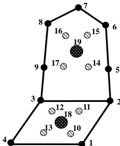
**Figure 3** Measurement locations - nine accelerometers were attached to seat frame and 10 accelerometers were attached to the seatback and seat cushion surfaces.
