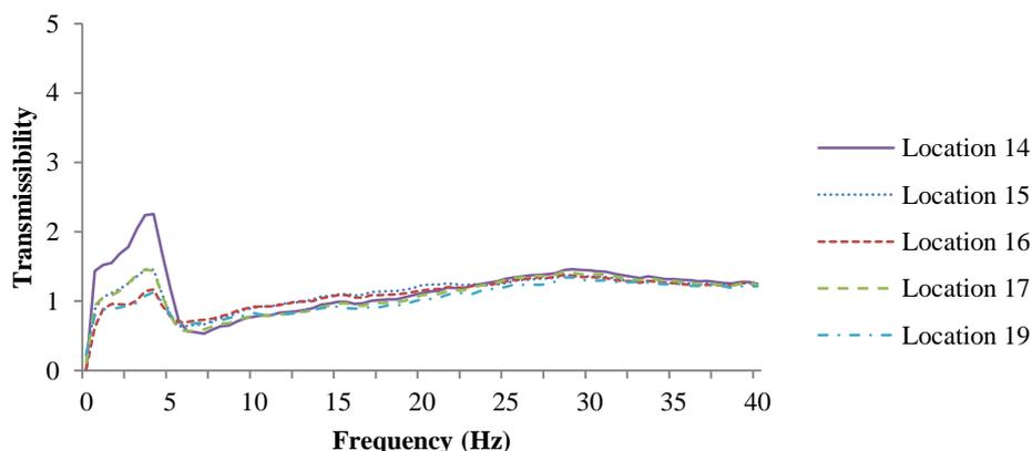
Figure 12 Vertical transmissibilities at measurement locations on seatback surface.
