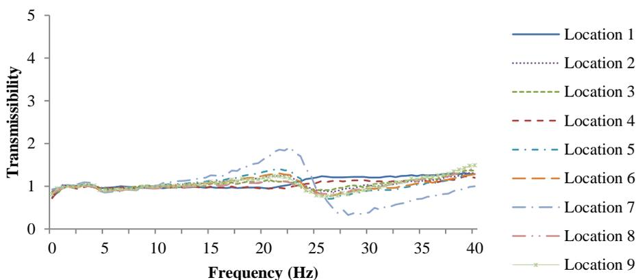
Figure 9 Vertical transmissibilities at measurement locations on seat frame
