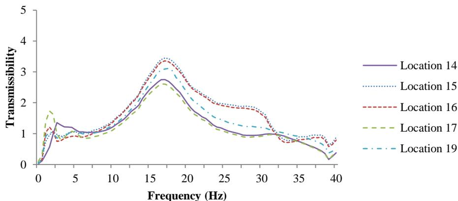
Figure 11 Lateral transmissibilities at measurement locations on seatback surface.
