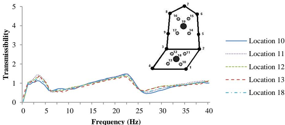
Figure 13 Fore-aft transmissibilities at measurement locations on seat cushion surface.
