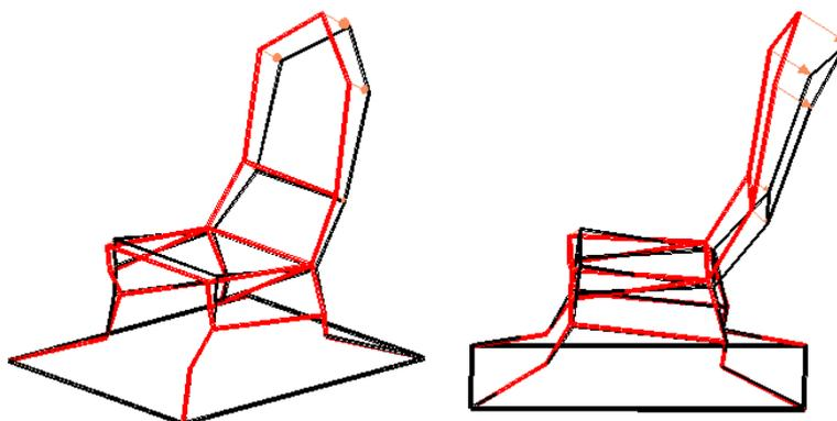
Figure 5 Fore-aft vibration mode shapes
