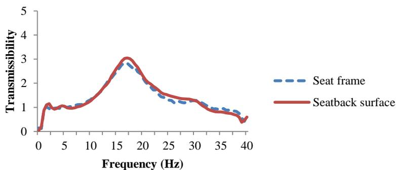
Figure 17 Average lateral transmissibilities on seatback frame and seatback surface.
