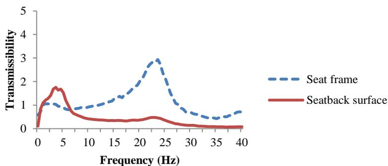
Figure 16 Average fore-aft transmissibilities on seatback frame and seatback surface.
