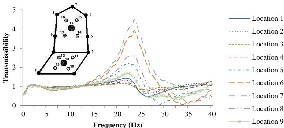
Figure 7 Fore-aft transmissibilities at measurement locations on seat frame
