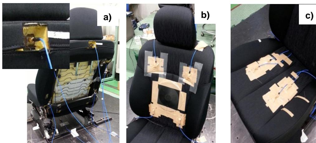
**Figure 2** Measurement locations a) tri-axial accelerometers on seat frame. b) Measurement locations on seatback surface with accelerometer pad and tri-axial accelerometers. c) Measurement locations on seat cushion surface with accelerometer pad and tri-axial accelerometers.
