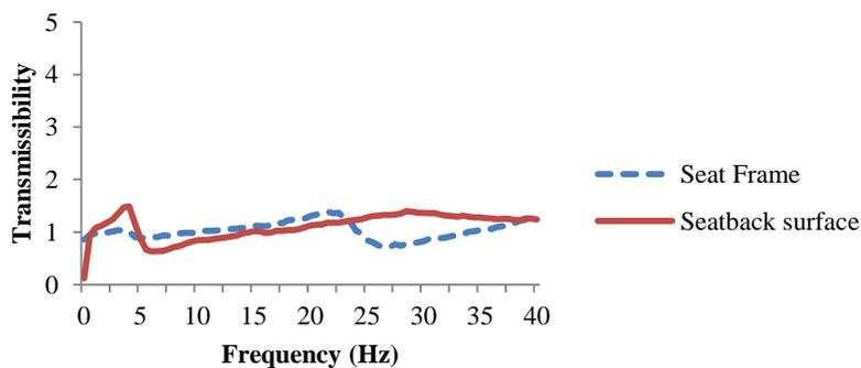
Figure 18 Average vertical transmissibilities on seatback frame and seatback surface.
