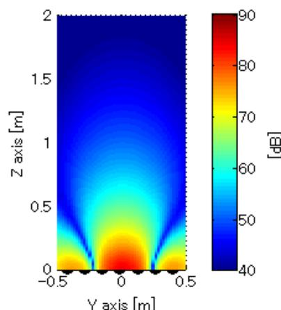
Figure 9 – Normalized sound pressure distribution of the speakers array at 100 Hz.
