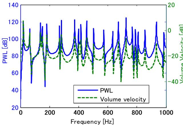
Figure 2 – Frequency characteristics of the acoustic power and volume velocity of the plate. (All odd mode)
