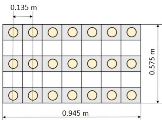
Figure 8 – Schematic diagram of a speakers array.
