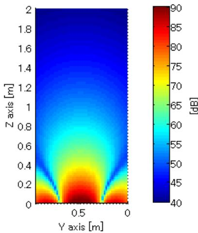
Figure 6 – Radiated sound pressure distribution from the plate at 77Hz. ( $m=1, n=1,3$ )
