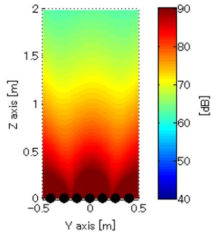
Figure 11 – Radiated sound pressure distribution from the speakers array at 400 Hz.
