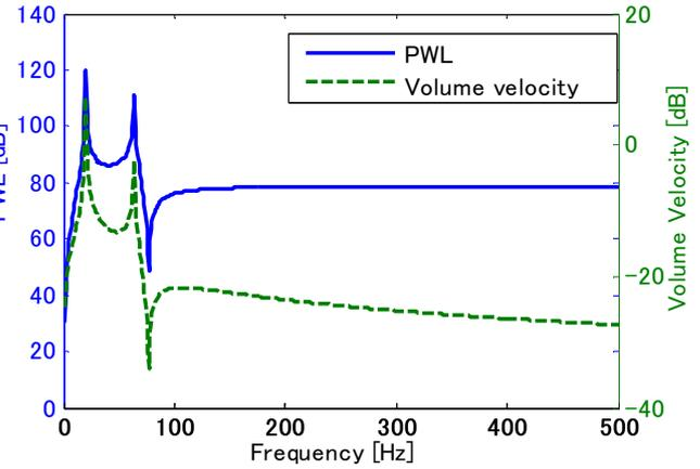
Figure 3 – Frequency characteristics of the acoustic power and volume velocity of the plate. ( $m=1, n=1,3$ )
