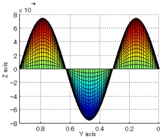
Figure 4 – Vibration displacement distribution at 64 Hz. (the (1, 3) mode)
