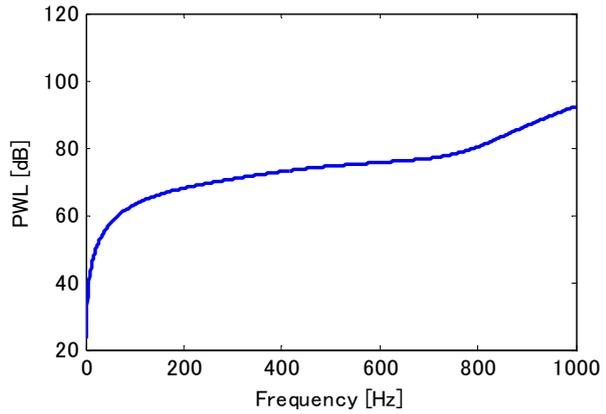
Figure 15 – Frequency characteristics of acoustic power of the speakers array. (the (1, 5) and the (1, 7) modes are coupled)
