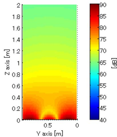
Figure 7 – Radiated sound pressure distribution from the plate at 77Hz. ( $m=1, n=3$ )
