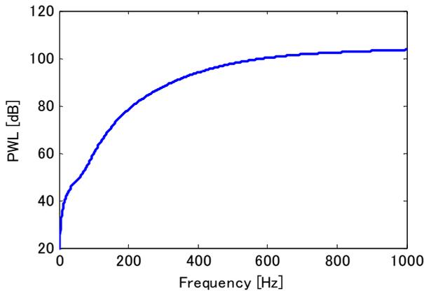
Figure 10 – Frequency characteristics of the acoustic power of the speakers array. (the (1, 1) and the (1, 3) modes are coupled)
