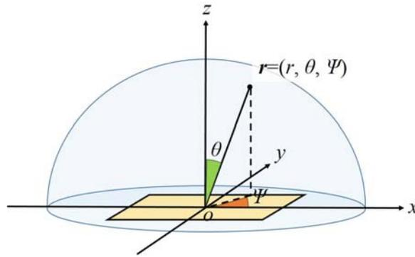
Figure 1 – Coordinate system in calculating the acoustic power of the rectangular plate.
