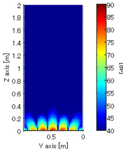
Figure 14 – Radiated sound pressure distribution from the plate at 470Hz. ( $m=1, n=5,7$ )
