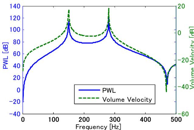
Figure 12 – Frequency characteristics of the acoustic power and volume velocity of the plate. ( $m=1, n=5,7$ )
