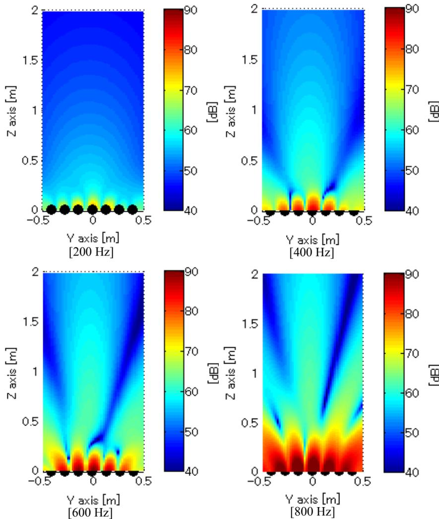
Figure 16 – Radiated sound pressure distribution from the speakers array.
