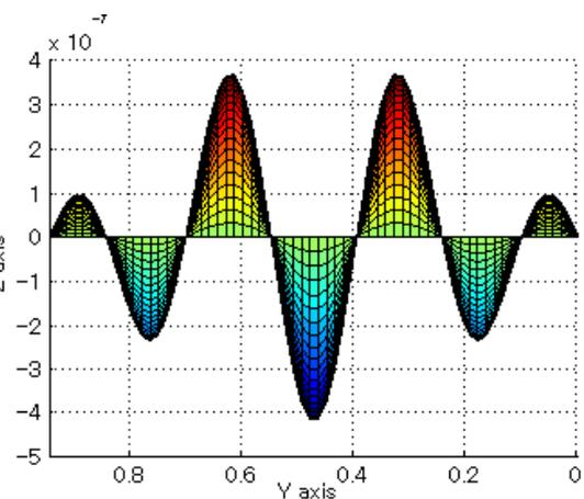
Figure 13 – Vibration displacement distribution at 460Hz. (the (1, 5) and the (1, 7) modes are coupled)
