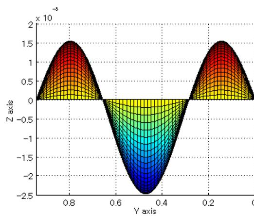
Figure 5 – Vibration displacement distribution at 77Hz. (the (1, 1) and the (1, 3) modes are coupled)
