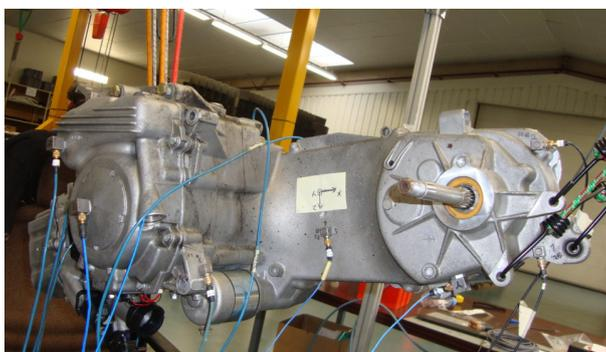
Figure 9 – Experimental modal analysis of the engine and casings of 125cc 4 strokes scooter
