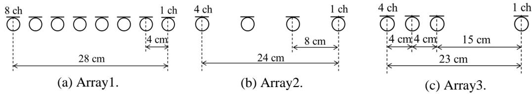
Figure 1 – The arrangement of microphone arrays.
