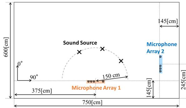
Figure 4 – Experimental arrangement.
