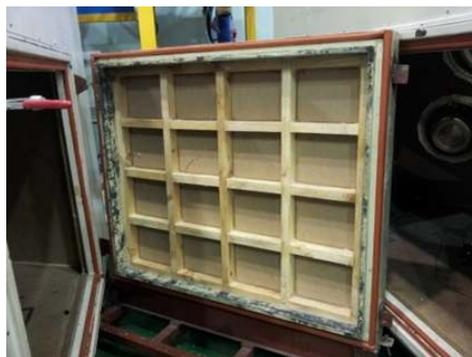
Figure 3. Stiffened panel with  $4 \times 4$  cells (205 mm x 255 mm)
