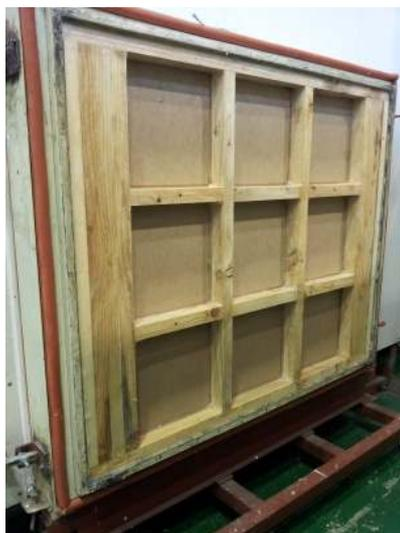
Figure 4. Stiffened panel with  $3 \times 3$  cells (280 mm x 280 mm)
