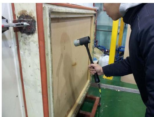
Figure 7. An impact hammer on the base material
