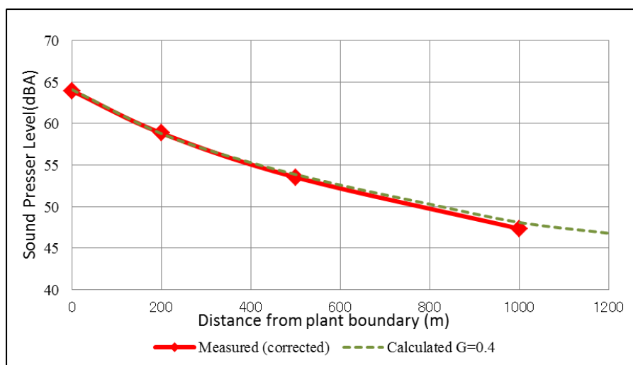
Figure 2 – Noise Attenuation on the desert by measurement and calculation
