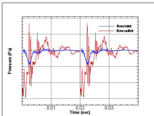
Figure 6 – Pressure at flow inlet and flow outlet
