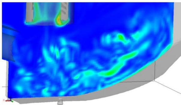
Figure 8 – Vorticity distributions inside main chamber of the muffler at 0.025097(sec)
