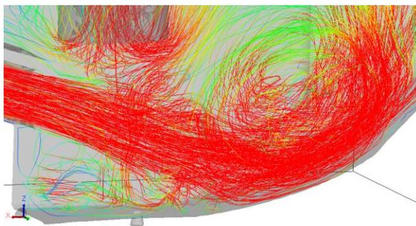
Figure 5 – Fluid stream lines with colored by velocity magnitude inside the main chamber of the muffler at 0.025097(sec)
