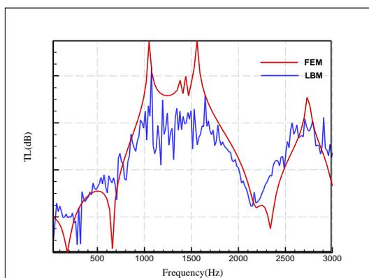
Figure 3 – Comparison of transmission loss between FEM and LBM
