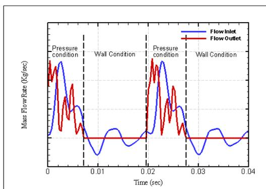
Figure 4 – Time-histories of mass flow rates computed at the inlet and outlet of flow
