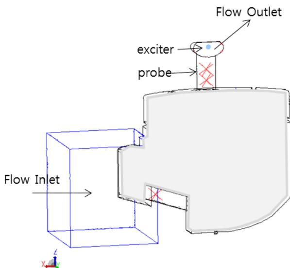
Figure 2 – Computational domain of suction muffler
