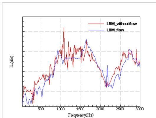
Figure 7 – Comparison of transmission loss between without flow and flow conditions
