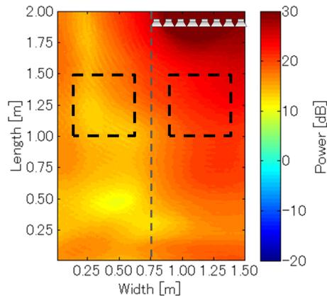
Figure 5 – Sound pressure distribution in unprocessed case.
