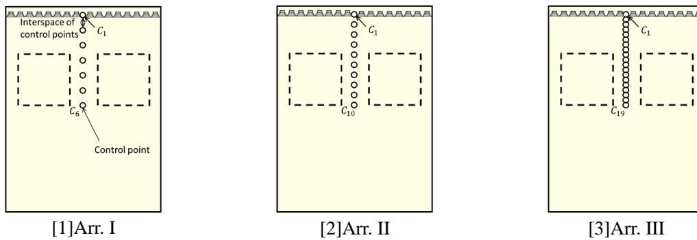
Figure 4 – The arrangement patterns of the NBSFC control points.
