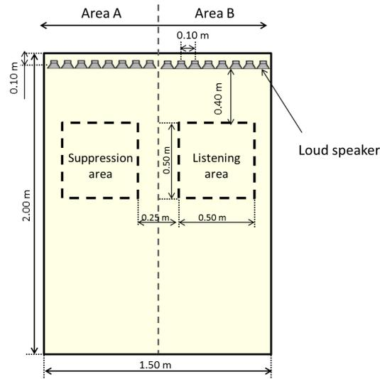
Figure 3 – Arrangement of the apparatus for numerical evaluation of the proposed method.
