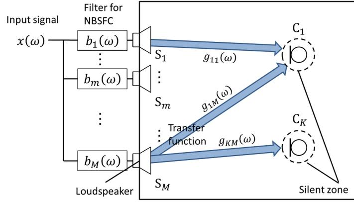
Figure 1 – Configuration of sound pressure suppression on each control points by NBSFC.
