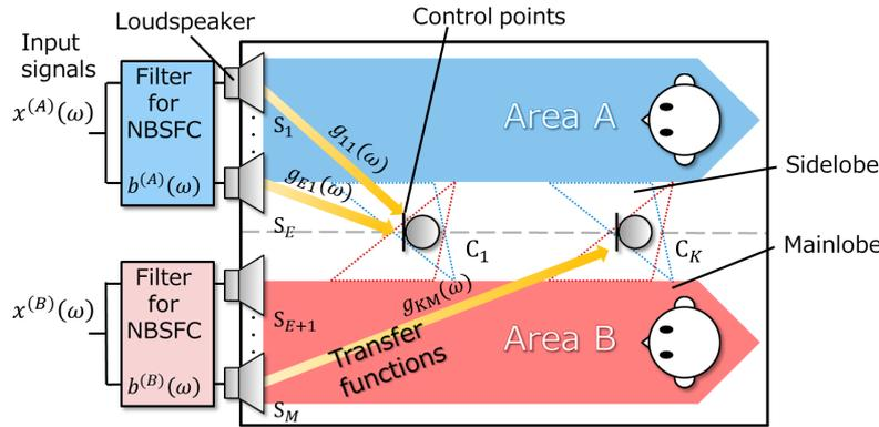
Figure 2 – Configuration of individual sound image generation for two users by the proposed method.
