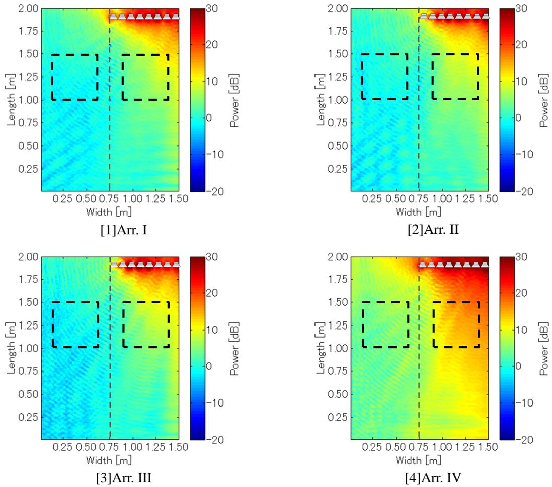
Figure 6 – Sound power distribution by each arrangement of control points.
