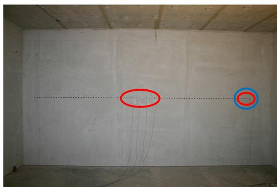
Figure 4 – Determination of the element attenuation by piezo transducers (**red**), excitation on the exterior side by a shaker (**blue**)
