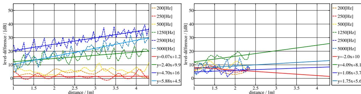
Figure 6 – Velocity level difference at different frequencies, horizontal (left) and vertical (right)
