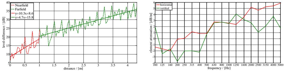
Figure 5 – Velocity level differences along the horizontal measuring path at 2500 Hz (left), element attenuation due to the internal damping (right)
