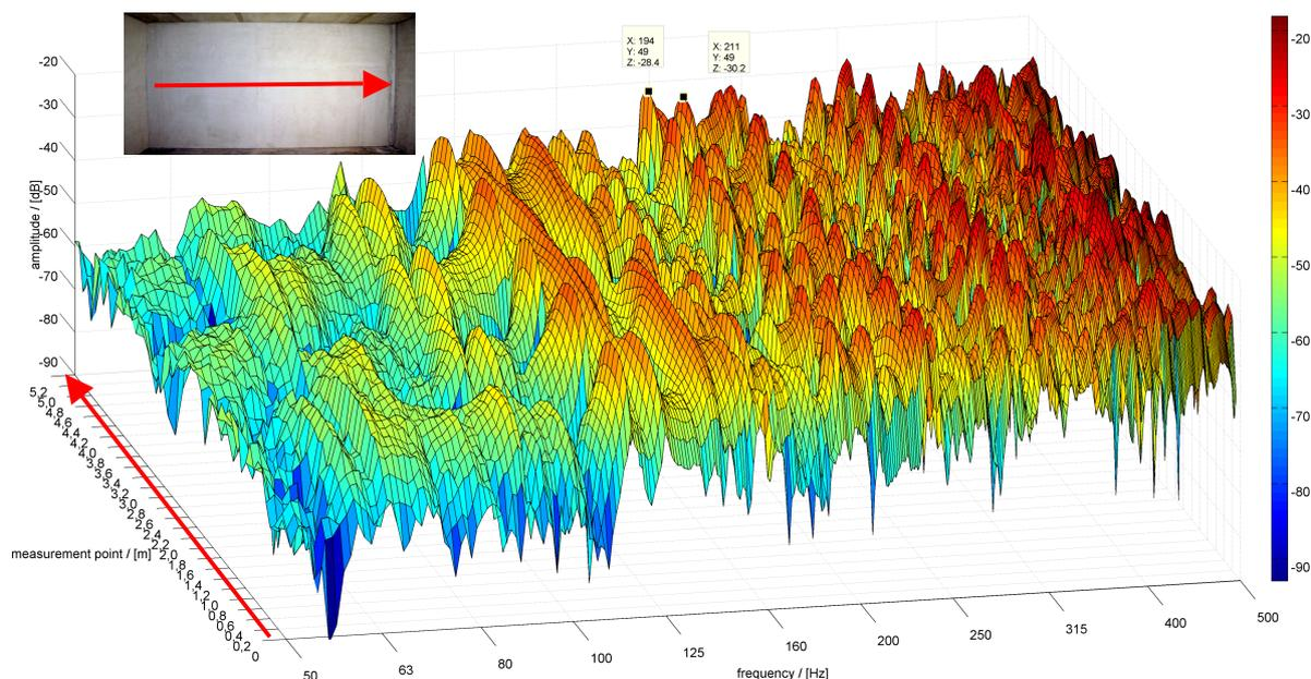
Figure 9 – Mode shapes of the entire wall on a horizontal measurement path
