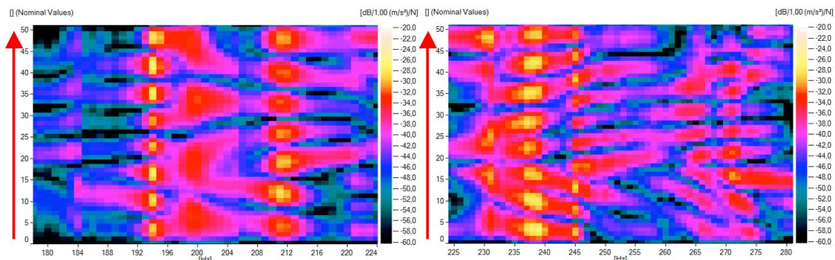
Figure 10 – Various ranges of mode shapes of the entire wall on a horizontal measurement path
