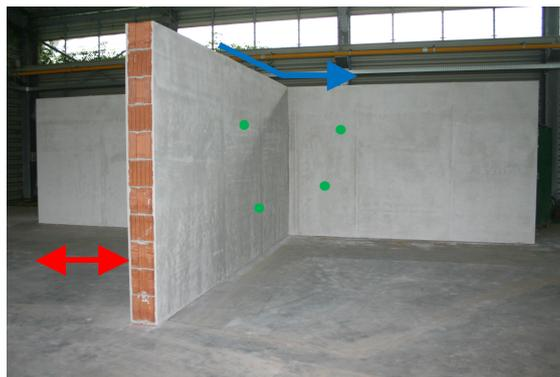
Figure 3 – T-junction of brickwork / measurement procedure: excitation of the wall by an electrodynamic shaker (**red**); determination of the velocity level by piezo transducer (**green**) to get the measurement values for the velocity level difference due to the junction (**blue**)
