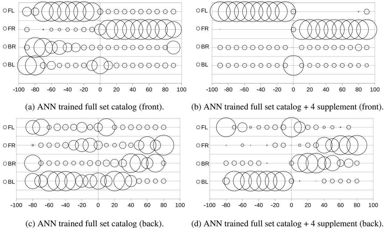
Figure 6: The front-back discrimination accuracy of FDBM implemented front-back discriminator in horizontal plane. Input signal is subset HRTF which is not used training of all ANN.
