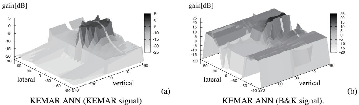
Figure 5: Directivity pattern obtained using the front-back discriminator trained by KEMAR HRTF catalog. The vertical axis shows normalized gain to the gain at  $(0^\circ, 0^\circ)$  and where -25 dB is used for flooring.
