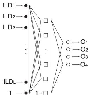
Figure 3: Structure of ANN. (●: Neurons of input layer, □: interlayer, ○: output layer.)
