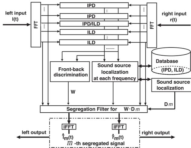
Figure 1: A block diagram of Frequency Domain Binaural Model with front-back discriminator.
