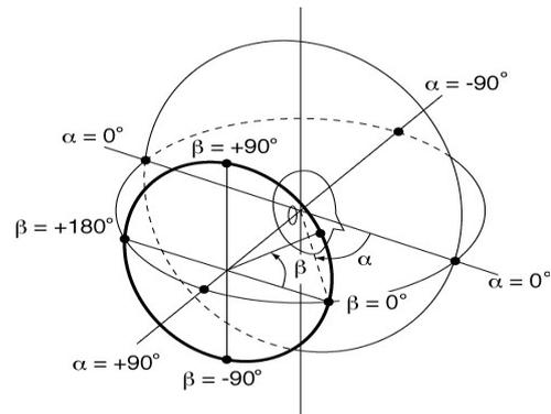
Figure 2: The sagittal coordinate system. A lateral angle :  $-90^\circ \leq \alpha \leq +90^\circ$ , and a vertical angle :  $-180^\circ \leq \beta \leq +180^\circ$ .
