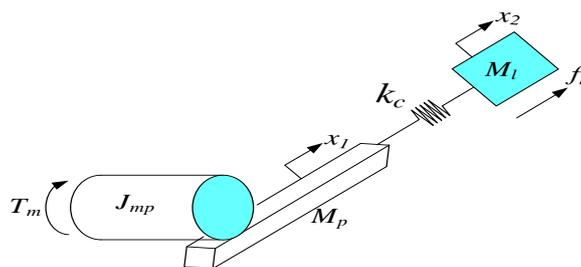
Figure 1 – The compliant actuator model with the rack pinion mechanism.
