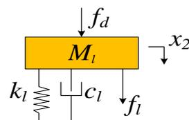
Figure 2 – The load mass with a spring-damper isolation system.
