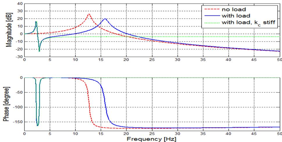
Figure 5 – Frequency responses  $rF_l(s)/T_m(s)$  for different compliant actuator systems.
