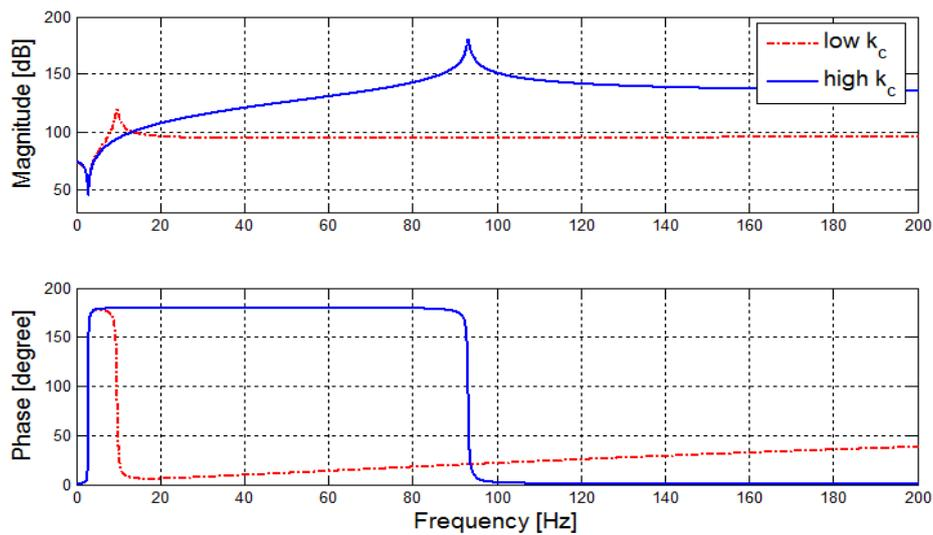
Figure 4 – Frequency response plot of  $F_l(s)/X_l(s)$  for varying compliant stiffness  $k_c$ .
