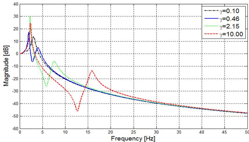
Figure 6 – Force transmissibility for a system using a compliant actuator: varying values of  $\gamma = k_c / k_l$ .
