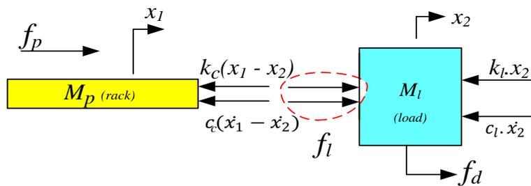
Figure 3 – Free body diagram of pinion's rack and load.
