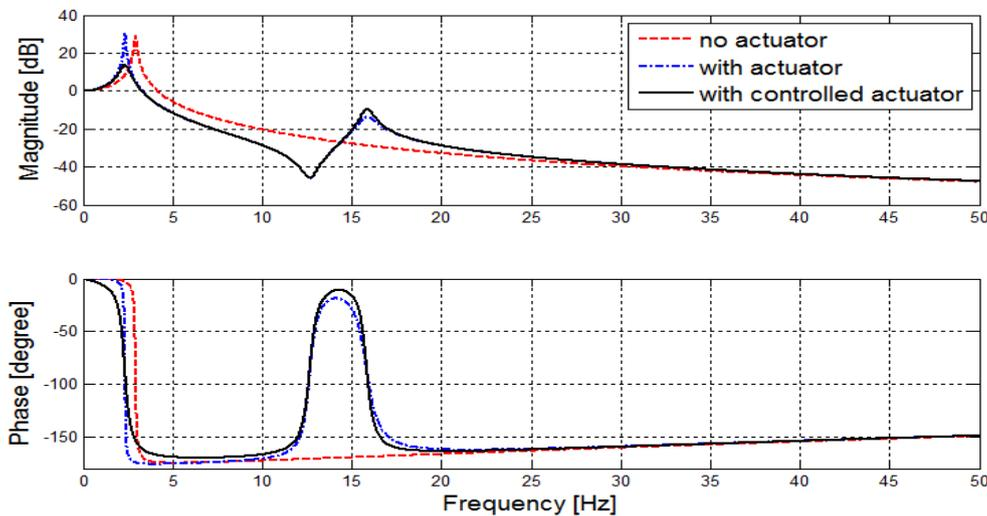
Figure 8 – Frequency response of  $F_t(s)/F_d(s)$  with and without the active control system.
