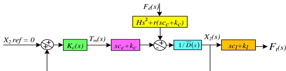
Figure 7 – The closed loop PD controller based on the position feedback.
