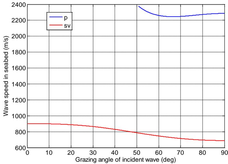
Figure 2 - Compressional wave and vertically polarised shear wave speeds in the seabed as a function of the grazing angle of the incident wave in the water column.
