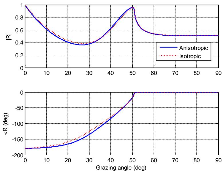
Figure 3. Magnitude and phase of the plane wave pressure reflection coefficient as a function of grazing angle for the anisotropic and isotropic seabed models discussed in the text.
