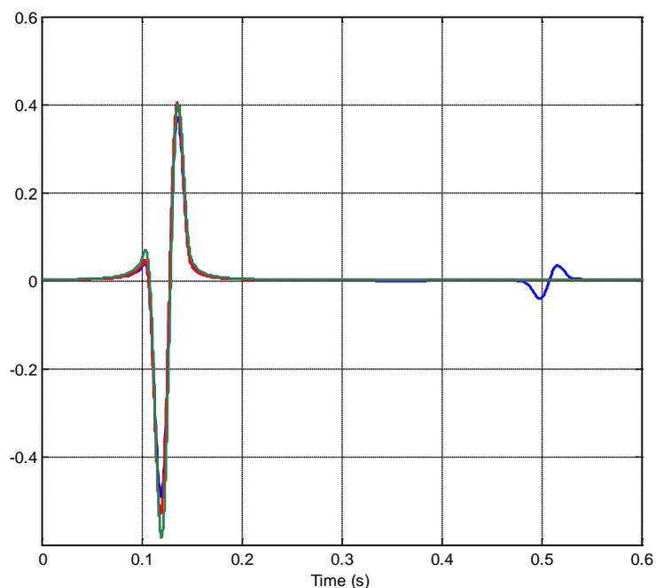
Figure 6. Waveform of reflected wave calculated by Fourier synthesis using numerically calculated reflection coefficients obtained from BOUNCE (blue), equivalent anisotropic seabed (Equation (7), red), and equivalent isotropic seabed (green).
