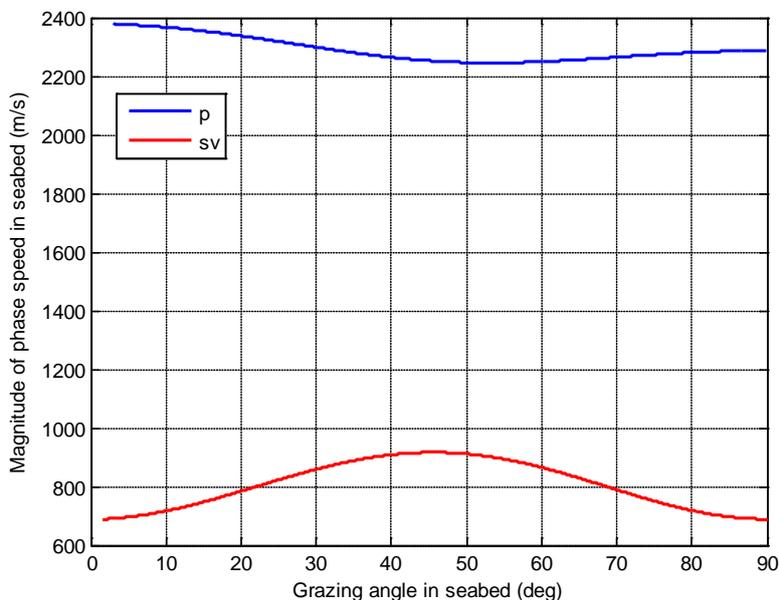
Figure 1. Compressional (*P*) and vertically polarised shear (*SV*) wave speeds as a function of the direction of the corresponding wave-vector in the seabed.
