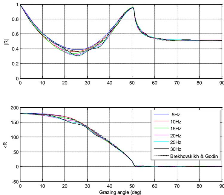
Figure 4. Magnitude and phase of the plane wave reflection coefficient computed by BOUNCE at the indicated frequencies for a seabed consisting of 100 repetitions of the two-layer sequence described in Table 1 over a halfspace with the isotropic medium properties described in the text, compared to the Brekhovskikh and Godin equivalent model given by Equation (7).
