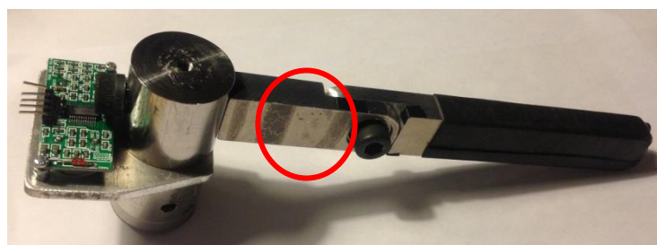
Figure 6- Mechanical design of the hand held impact hammer device – the circle shows the hinge allowing near-free fall of the hammerhead
