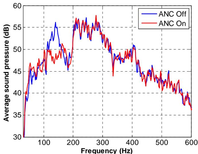
Figure 6 - Spatially averaged engine noise spectra with and without the global active noise control.
