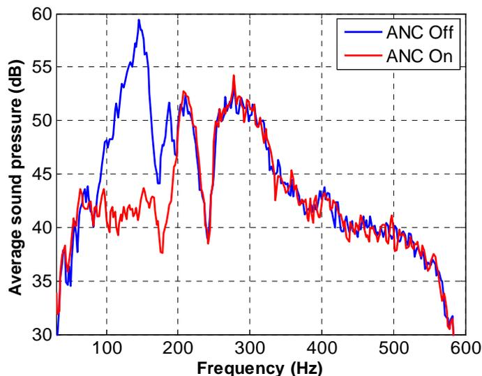
Figure 5 - Noise spectra from one of the error microphones of global active control system
