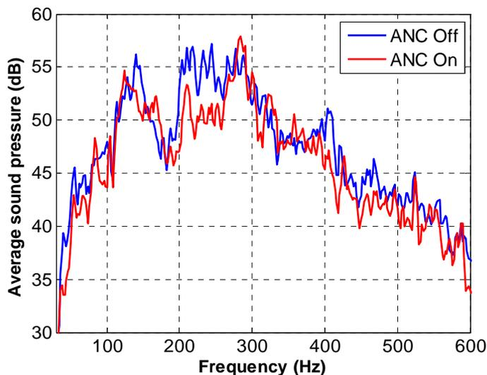
Figure 8 - Spatially averaged engine noise spectra with and without active control at the open ends.
