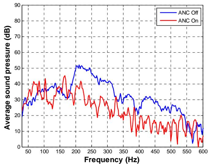
Figure 7 - Noise spectra from one of the error microphones of the duct active control system
