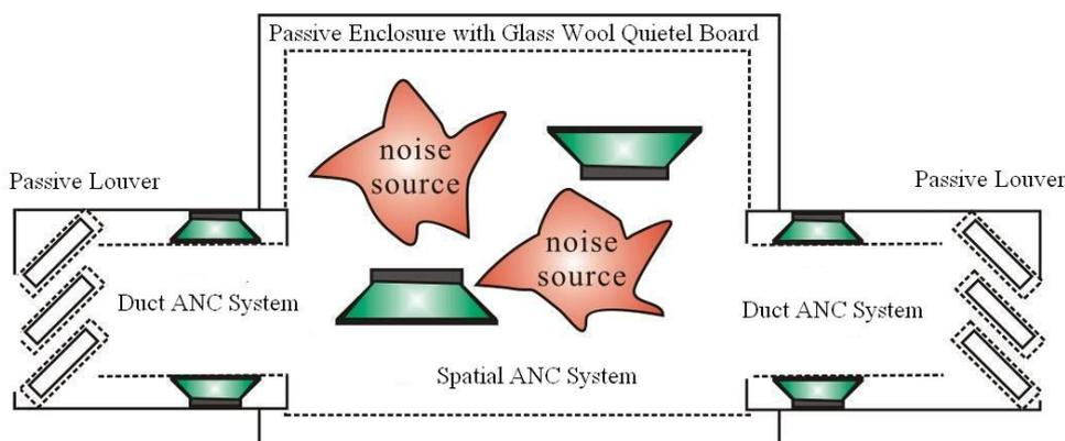
Figure 1 – Schematic diagram of the integrated passive and active enclosure.
