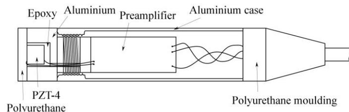
Figure 1 – Construction of an ITC8257 hydrophone.
