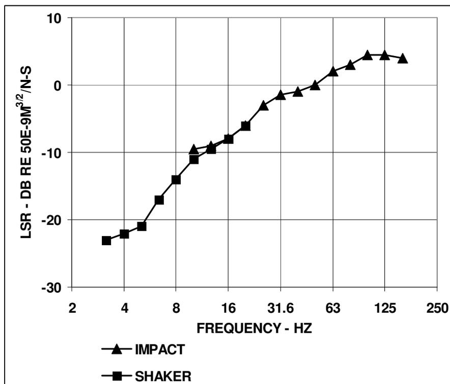
Figure 3. Comparison of Impact and Shaker LSR Test Result
