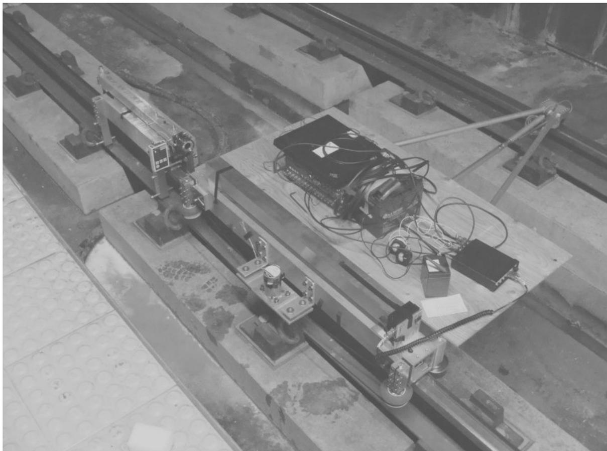
**Figure 6. Rail Undulation Measurement**
