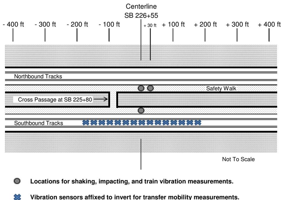
Figure 2. Schematic of Tunnel Test Set-Up
