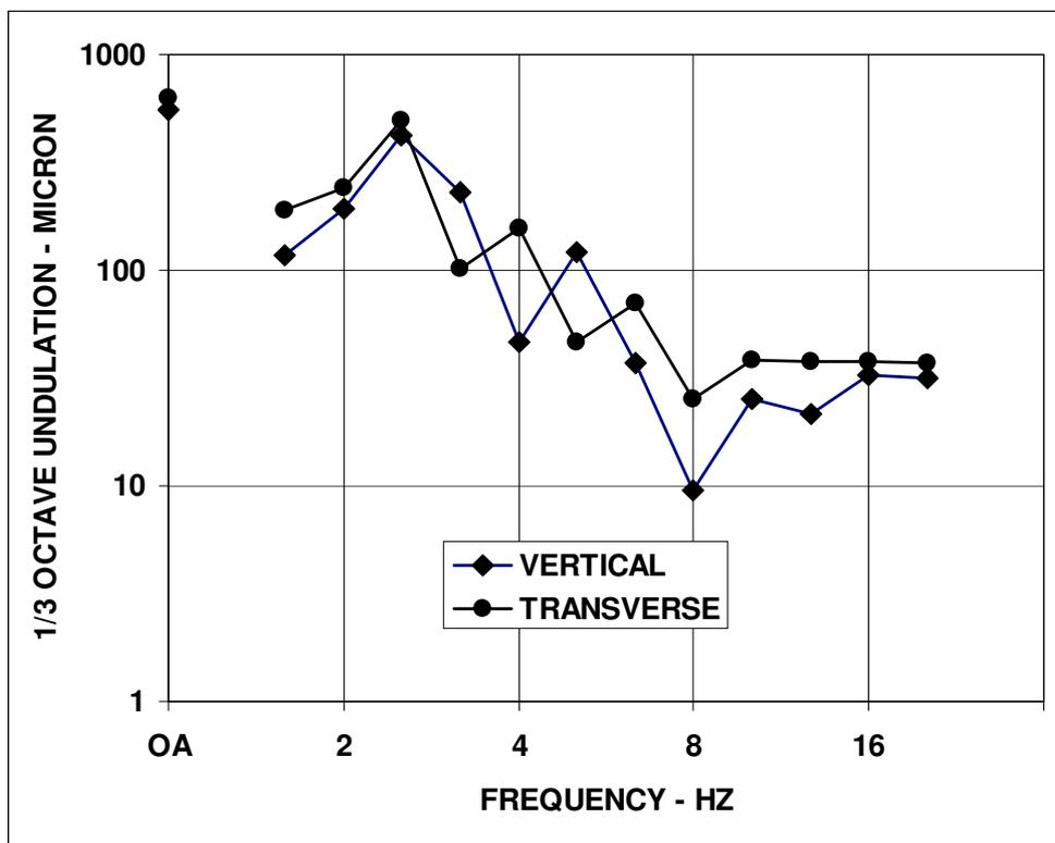
Figure 8. Equivalent Rail Vibration Displacement at 48km/h
