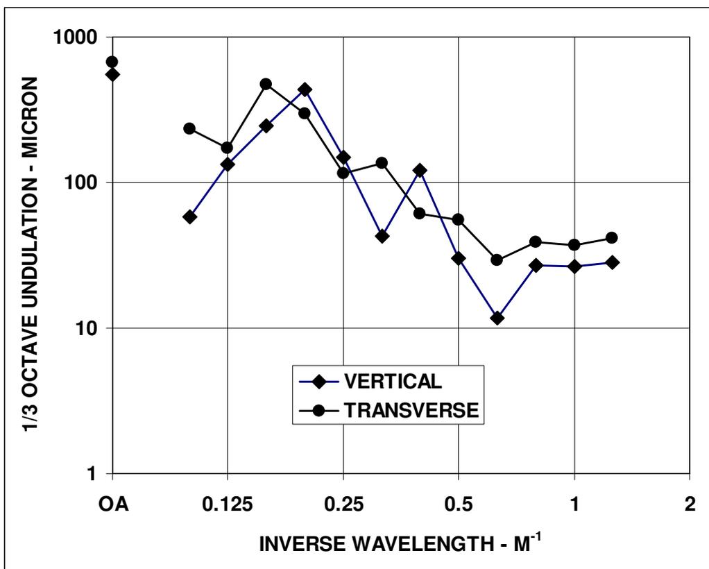
Figure 7. Rail Undulation versus Inverse Wavelength
