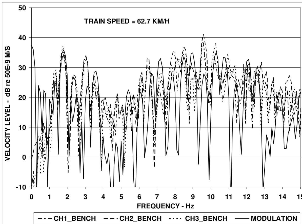
Figure 9 Comparison of tunnel bench vibration with modulation spectrum
