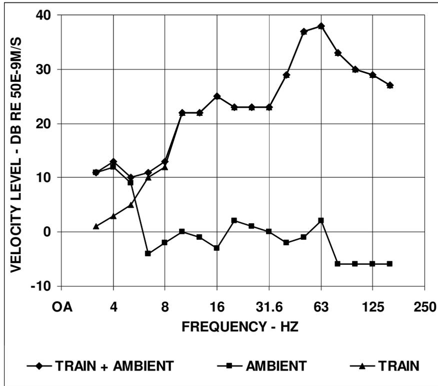
Figure 4. Tunnel Bench Vibration Velocity at 40km/h
