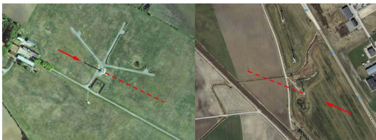
**Figure 2: The T1 (left) and V27 turbine (right) with surroundings. Wind direction (red arrow) and microphone placement line (dashed). Upwards is north. <sup>6</sup>**
