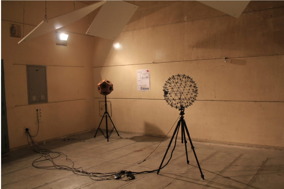
Figure 2 – Measurement setup: microphone array and dodecahedron in the reverberation chamber.
