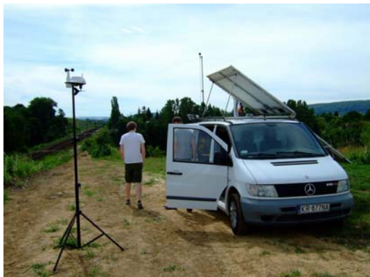
Figure 2 - The mobile station of long-term acoustic monitoring (exterior view)
