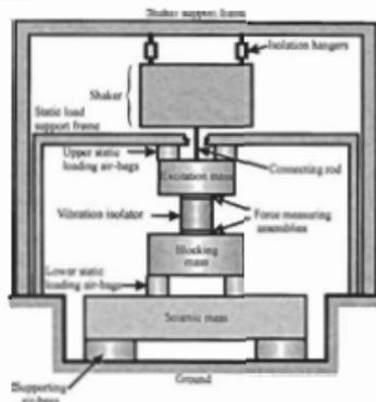
Figure 4: Schematic diagram of vibration isolator test rig.
