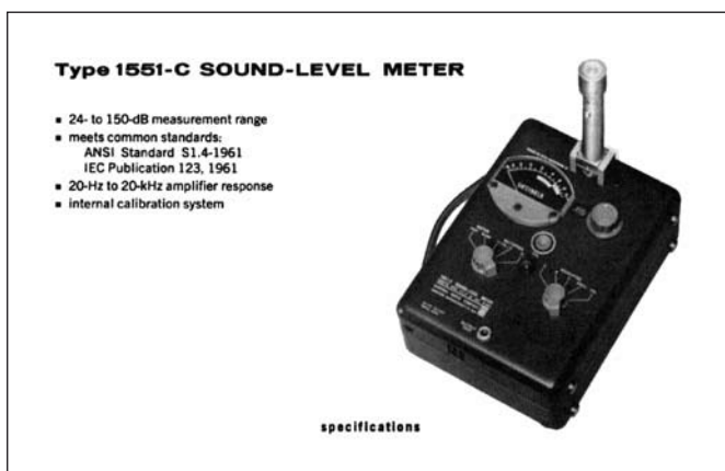
Fig 2. An early sound level meter used by the author [GenRad 1963]
