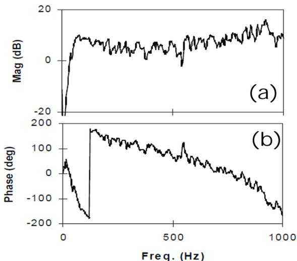
Figure 3 Magnitude (a) and phase (b) of the measured open-loop frequency response of the uncompensated system in Example 1.
