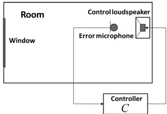
Figure 1 Schematic of the feedback control system.
