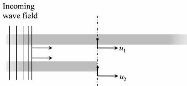
**Figure 7.** Schematic showing an infinite bar (upper) and semi-infinite bar (lower) subjected to an equivalent pressure wave field and the respective displacements at the boundary of the semi-infinite bar
