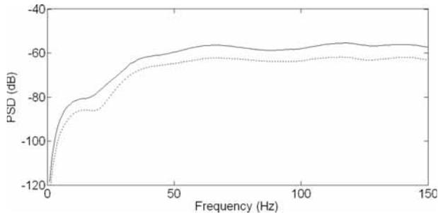
Figure 5. Response at  $x=10\text{m}$  for a tunnel depth of 5m: (solid-line)-PiP v4 with free-surface; (dotted-line)-PiP v3 using fullspace solution; results presented in dB (ref  $1\text{ mm}^2/\text{Hz}$ )
