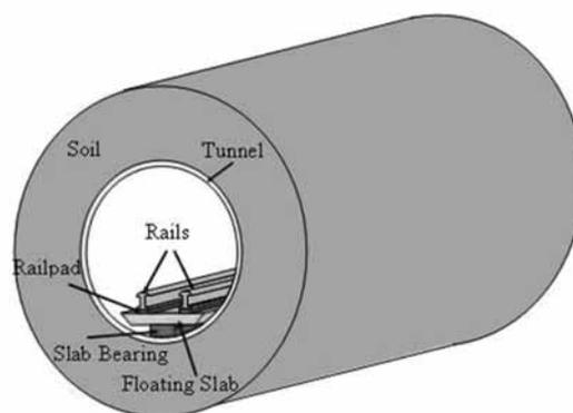
Figure 1. A floating-slab track coupled to the tunnel-soil model
