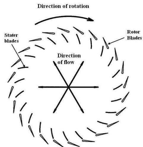
Figure 3. Rotor and stator blades in the Mupod.
