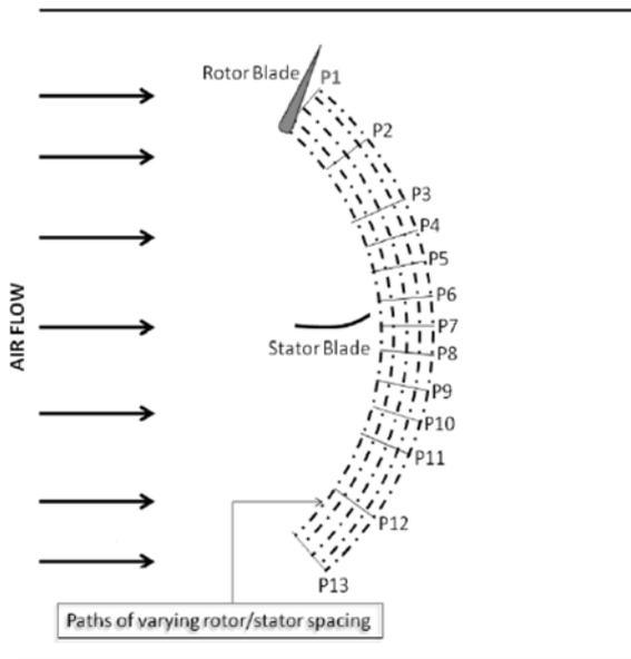
Figure 7. Rotor blade positions for surface pressure measurement.
