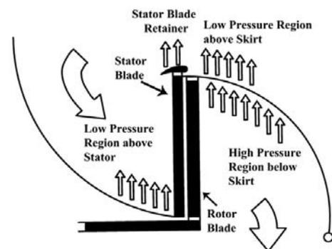
Figure 2. Illustration diagram of lift generation in the cross section of the Mupod.
