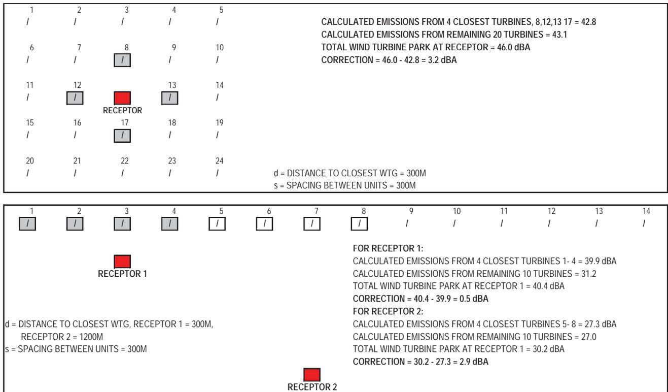
Figure 7. Computation results of correction C for use in equation (1)
