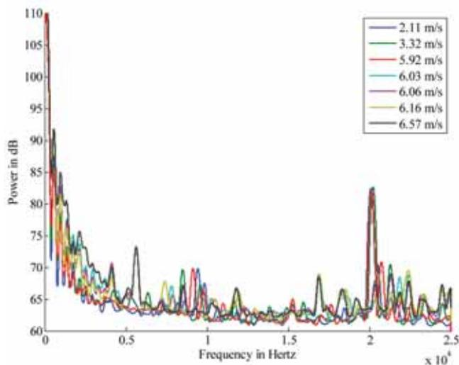
Figure 2(a). Power spectral density for various wind speeds using the Bartlett Method
