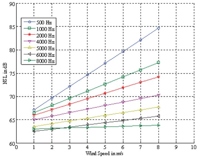
Figure 3. Effect of NSL at different wind speeds for different frequencies
