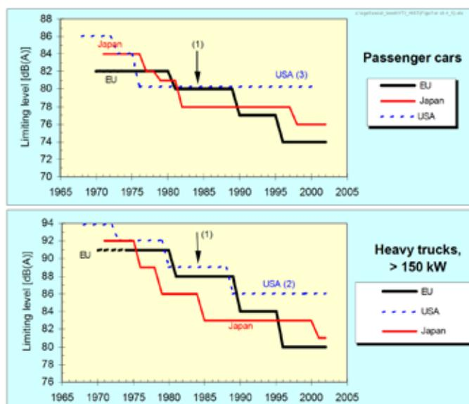
Figure 2. Examples of the development of individual vehicle noise emission limits over the years including some projected limits [7]
