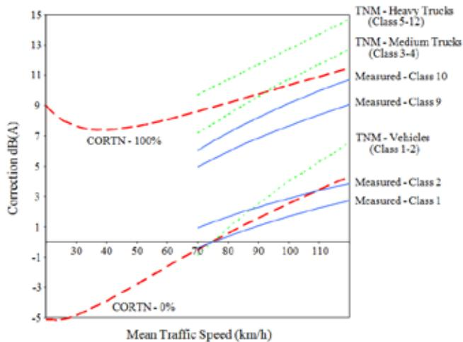
Figure 1. Correction to traffic noise emissions levels using TNM, CORTN and measured by Jurevicius et al. [7] with varying percentage commercial vehicles (normalised to 75 km/hr and 0% commercial vehicles)
