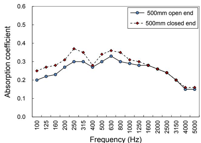
Figure 4. Measured results of the rectangular MPP space absorbers (RMSAs) of 500 mm x 500 mm square section. Solid line: open top ends; Dashed line: closed top ends with covers
