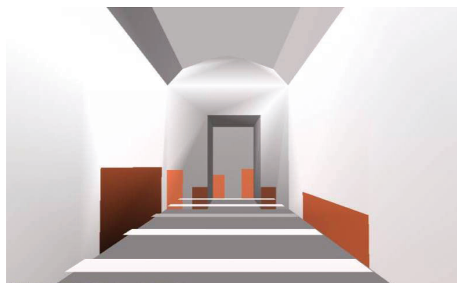
Figure 8. Render of 3D virtual model by Odeon with the absorbent panels insertion on the walls
