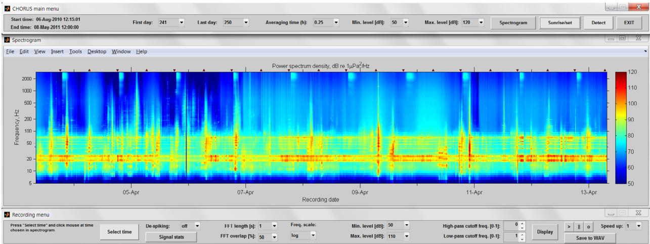
Figure 1: LTA spectrogram of sea noise recorded for 10 days compiled from PSDs of individual recordings. The red upward and downward triangles indicate the sunrise and sunset time respectively.
