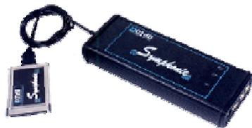
Together with a Windows-based dedicated software, PRO-515 allows easy and reliable measurement of the acoustic absorption "α" coefficient of porous materials.
