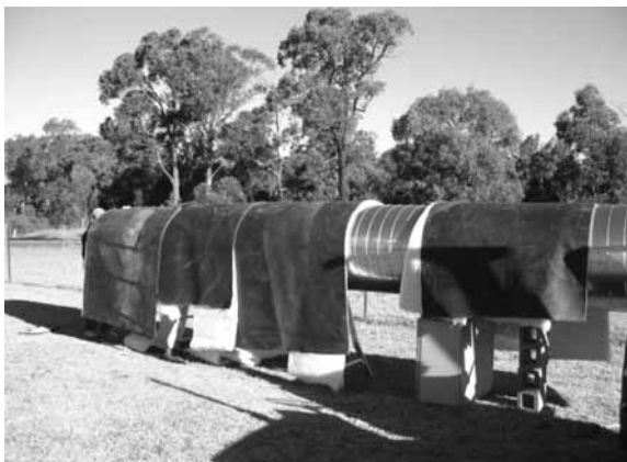
Source: Daniel Potente Figure 6. Loaded vinyl wrapped 915 mm duct
