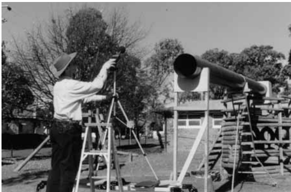
Source: Murray Neish Figure 5 Murray Neish Testing a 400 mm Duct
