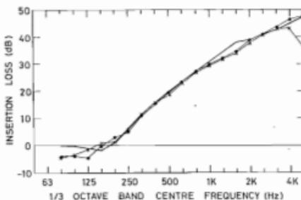
Figure 8: Predicted and measured 1/3 octave band insertion losses for "typical" lagging. Measured values with final rig configuration. — Theoretical values. — Derived from measured intensities. — Derived from measured pressures.
