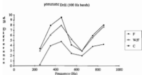
Figure 3: Relative radiated sound power levels (dB difference) for the pneumatic hand drill. (F — difference between floor and free space values; W/F — difference between wall/floor intersection and free space values; C — difference between corner and free space values.)
