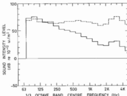
Figure 6: Space averaged sound intensity measurements with final rig configuration. — Bare plate. — With "typical" lagging.
