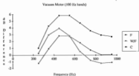
Figure 2: Relative radiated sound power levels (dB difference) for the vacuum cleaner motor. (F — difference between floor and free space values; W/F — difference between wall/floor intersection and free space values; C — difference between corner and free space values.)
