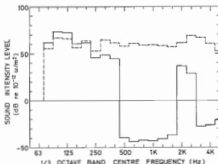
Figure 3: Space averaged sound intensity measurements with initial rig configuration. — Bare plate. — With "typical" lagging.
