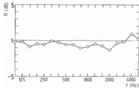
Figure 6: Deviation of the sound transmission loss of the 6 mm thick glass panel with absorbing material from the values without absorbing material in the niche
