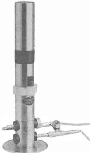
Fig. 3. Pistonphone placed on coupler for sound intensity and particle velocity calibrations.
