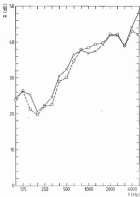
Figure 7: Comparison of the sound transmission loss of a double (4/12/10) mm glass panel:
