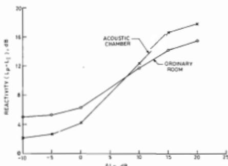
Figure 2: Reactivity vs background and source sound pressure level difference,  $\Delta L_p$ .
