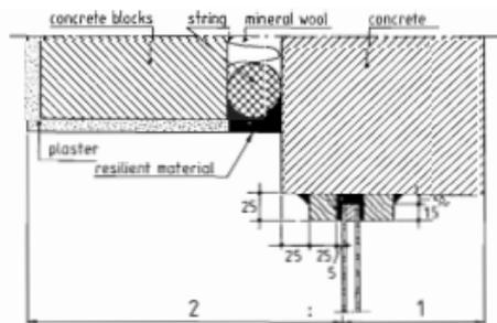
Figure 2: Mounting of the test specimen on the staggered opening, following DIN 52 210 (dimensions in mm)
