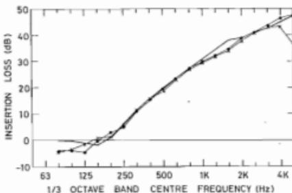
Figure 8: Predicted and measured  $\frac{1}{3}$  octave band insertion losses for "typical" lagging. Measured values with final rig configuration. — Theoretical values. — Derived from measured intensities. — Derived from measured pressures.
