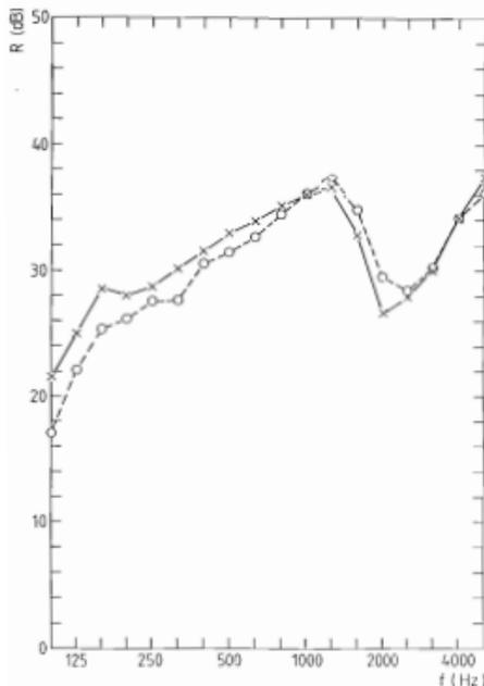
Figure 10: Comparison of the sound transmission loss of the PVC-window with a glass panel of thickness 6 mm:
