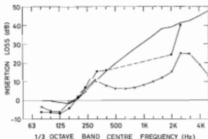
Figure 5: Predicted and measured 1/3 octave band insertion losses for "typical" lagging. Measured values with initial rig configuration. — Theoretical values. — Derived from measured intensities. — Derived from measured pressures. [— — — Associated with negative intensity with lagged plate].
