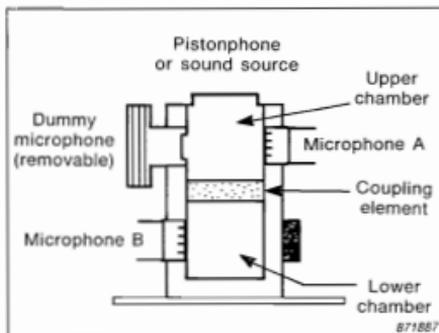
Fig. 2. Simplified cross section of intensity coupler.
