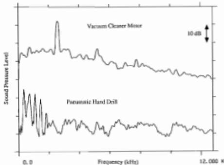
Figure 1: Sound pressure level spectra of the vacuum cleaner motor and the pneumatic hand drill (relative units, dB re  $2 \times 10^{-5}$  Pa)
