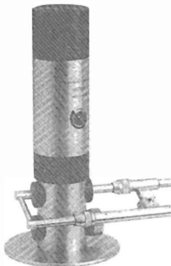
Fig. 4. Broadband source placed on coupler for measuring residual intensity and residual pressure-intensity index.
