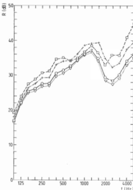
Figure 9: Sound transmission loss of the PVC window obtained with the intensity method (probe distance 5 cm):
