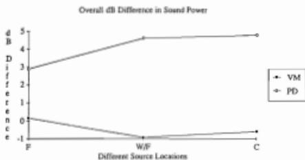
Figure 4: Relative overall radiated sound power levels (dB difference) for the vacuum cleaner motor (VM) and the pneumatic hand drill (PD) for different source locations.
