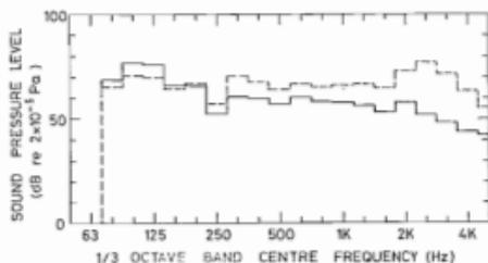
Figure 4: Space averaged sound pressure measurements with initial rig configuration. — Bare plate. — With "typical" lagging.
