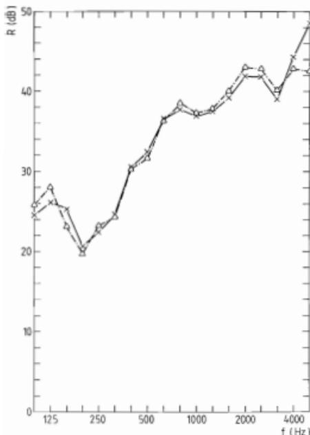
Figure 8: Comparison of the sound transmission loss of a double (4/12/10) mm glass panel:
