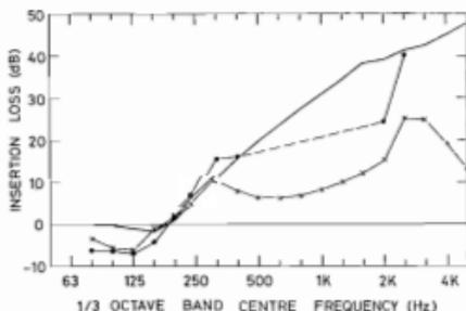
Figure 5: Predicted and measured  $\frac{1}{3}$  octave band insertion losses for "typical" lagging. Measured values with initial rig configuration. — Theoretical values. — Derived from measured intensities. — Derived from measured pressures. [— — — Associated with negative intensity with lagged plate].
