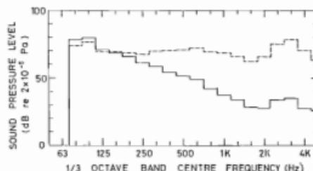
Figure 7: Space averaged sound pressure measurements with final rig configuration. — Bare plate. — With "typical" lagging.
