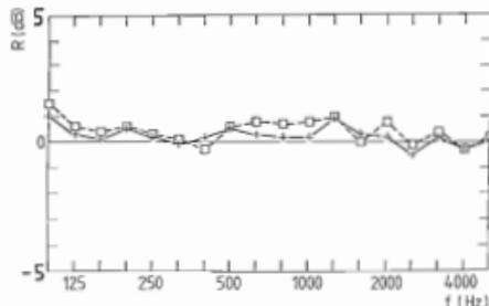
Figure 3: Deviation of the sound transmission loss results obtained with the scanning method from the fixed points method:
