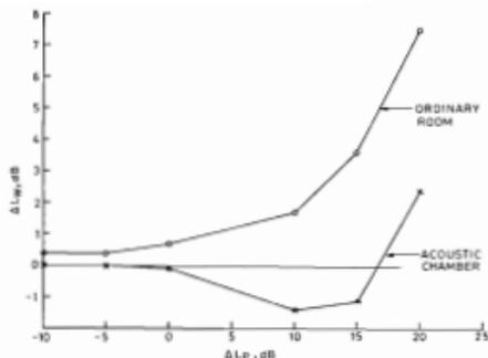
Figure 1: Influence of the difference of background and source noise level,  $\Delta L_p$ , on the accuracy of sound power determination.
