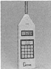
The Cirrus CRL 702 Data Logging Sound Level Meter
