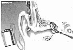
Figure 1. A diagram of the Nucleus implantable receiver-stimulator and wearable speech processor unit for clinical trial by the FDA illustrating the components. Speech is picked up by the directional microphone and electrical signals sent to the speech processor for coding. The coded signals and power to operate the implant are transmitted through the intact skin by radio waves (inductive coupling). The implant decodes the signals and directs them to the electrodes in the array lying around the basal turn of the inner ear.
