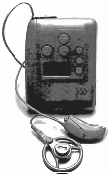
The Sprint™ advanced speech processor, which is the external part of Cochlear's new System 24™ cochlear implant hearing system.
