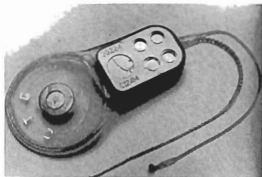
The C124M™ implanted receiver-stimulator and flexible electrode array which is the heart of the System 24™ cochlear implant hearing system produced by Cochlear. This system is able to provide higher rates of stimulation, monopole stimulation, and a telemetry function.
