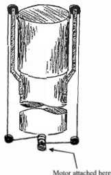
Figure 5. Exhaust stack with an adjustable sleeve to minimise the noise radiated from the top of the stack.
