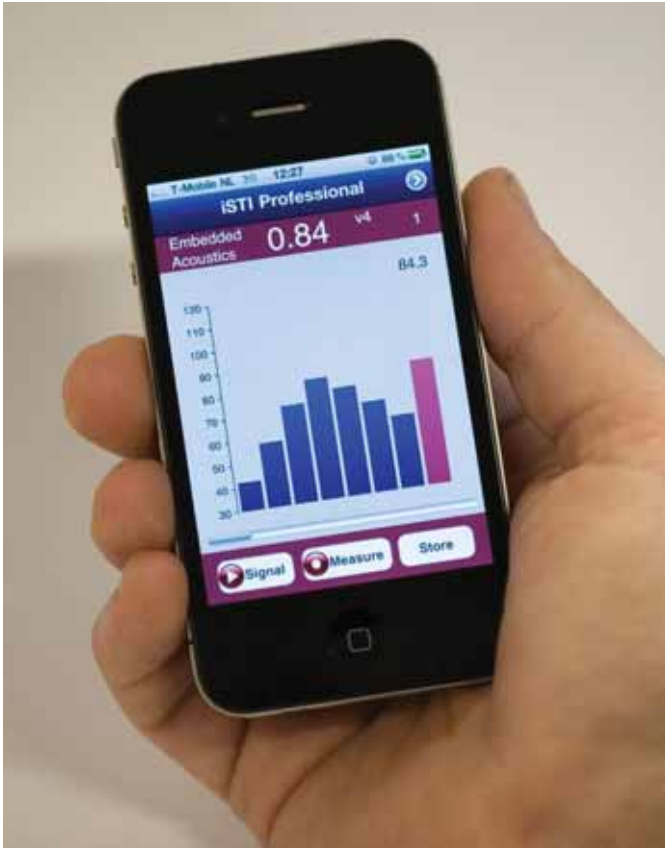
Figure 4. iPhone apparatus for performing 4th edition-compliant STIPA measurements (2011)
